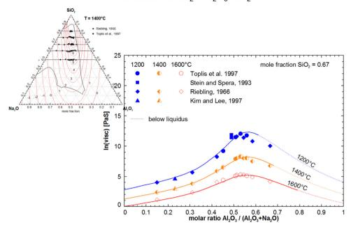
Fig. 19. Viscosity module - viscosities in Na<sub>2</sub>O-Al<sub>2</sub>O<sub>3</sub>-SiO<sub>2</sub>.
