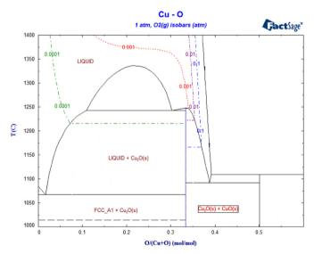
Fig. 34. Phase Diagram module – calculated  $O_2(g)$  isobars in the Cu–O binary systems using data from FScopp.
