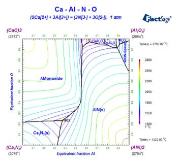
**Fig. 25. Phase Diagram** – polythermal liquidus projection in the Ca<sub>3</sub>N<sub>2</sub>–Al<sub>2</sub>O<sub>3</sub>–CaO–AlN reciprocal system using data from **FTOxCN**.
