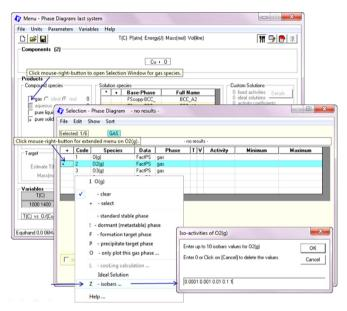
**Fig. 33. Phase Diagram** module – isobars and iso-activity lines for compound species are defined in the *Compound Selection Window*.
