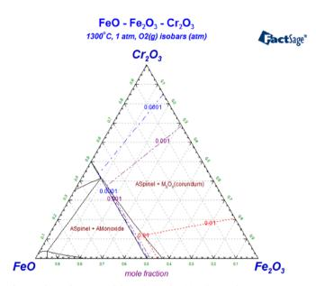
Fig. 35. Phase Diagram module – calculated  $O_2(g)$  isobars in the FeO–Fe<sub>2</sub>O<sub>3</sub>–Cr<sub>2</sub>O<sub>3</sub> ternary system at 1300 °C using data from **FToxid**.
