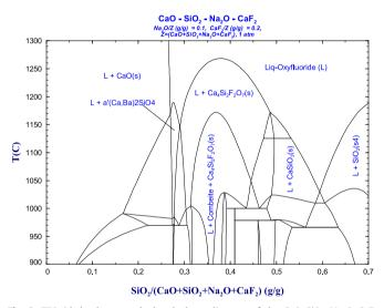
Fig. 3. FTOxid database – calculated phase diagram of the  $CaO-SiO_2-Na_2O-CaF_2$  system.
