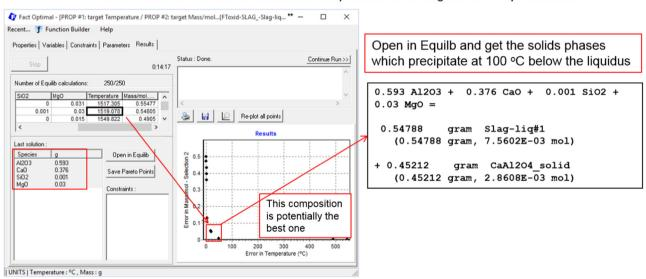
Fig. 18. FactOptimal module – Results Window to minimize simultaneously the liquidus temperature and solid mass fraction in the in the Al<sub>2</sub>O<sub>3</sub>–CaO–SiO<sub>2</sub>–MgO oxide system.
