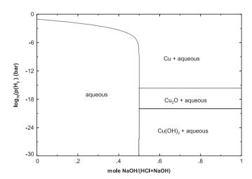
Fig. 38. Phase Diagram – calculated partial pressure of  $H_2$  vs. molar ratio NaOH/(NaOH+HCl) for the the system  $H_2O$ -Cu-NaOH-HCl-H<sub>2</sub>, molality of Cu=0.001.
