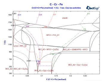
**Fig. 36. Phase Diagram –** calculated C(s) iso-activity lines in the Fe–Cr–C ternary system.
