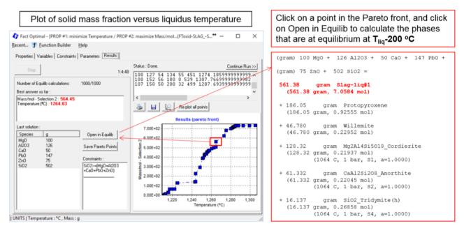
Fig. 17. FactOptimal module – results showing the Pareto front in a plot of solid fraction vs. liquidus temperature in the MgO-Al<sub>2</sub>O<sub>3</sub>-CaO-PbO-ZnO-SiO<sub>2</sub> oxide system.
