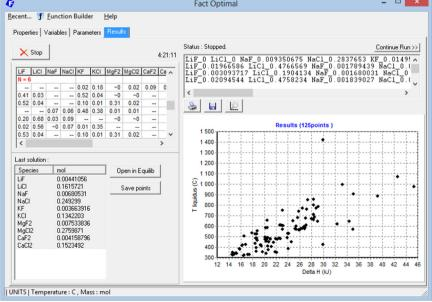
Fig. 16. FactOptimal module - calculated of characteristic points in the Li+, Na+, K+, Mg++, Ca++ / F-, Cl- reciprocal system.
