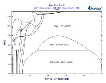
**Fig. 29. Phase Diagram** – T(K) vs. Cr/(Fe+Cr) phase diagram of the Fe-Cr-C-N system at C/(Fe+Cr)=0.02 and N/(Fe+Cr)=0.02 calculated under normal equilibrium conditions (orthoequilibrium) using data from **FSstel**.
