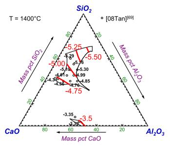
**Fig. 37. Phase Diagram** – calculated iso-sulfide capacity ( $C_S$ ) lines of CaO–SiO<sub>2</sub>– Al<sub>2</sub>O<sub>3</sub> slag at 1400 °C with the calculated liquidus (thin lines) [25] using data from **FToxid**.
