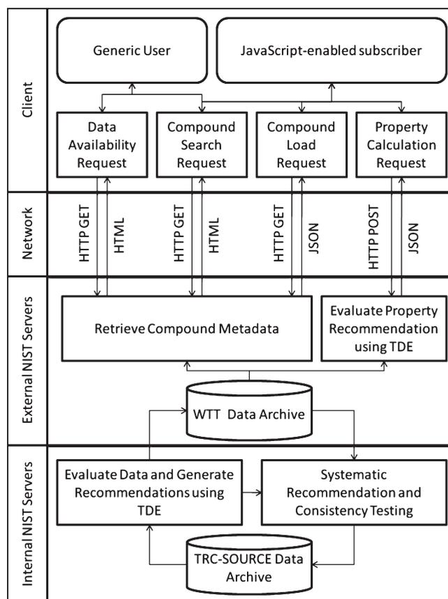
Figure 1. Schematic of data flow through the application stack.
